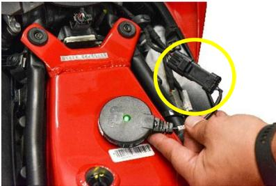
**ENG** Connect the UpMap cable provided to the bike's diagnostics connection port (generally located under the seat) and proceed with the installation, following device instructions
